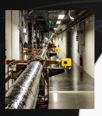
Here, in the electron gun, the electrons are accelerated to a speed close to that of light.
