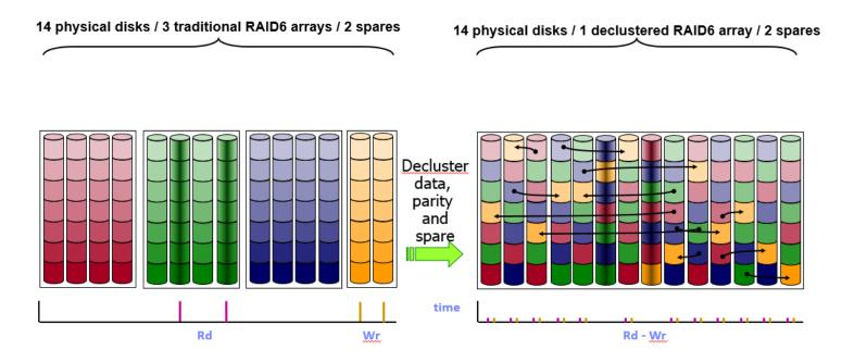
Rebuild activity confined to just a few disks – slow rebuild, disrupts user programs Rebuild activity spread across many disks, less disruption to user programs
