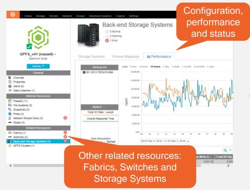
Clusters may use NSDs built off of SAN attached storage such as FlashSystems or other block storage systems. Latency within the Spectrum Scale file system may be due to issues within the storage or the fabric connections.
