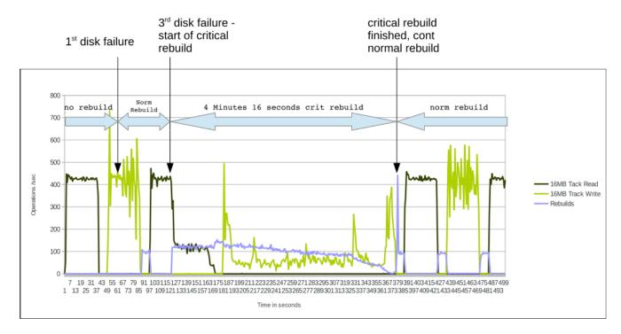
As one can see during the critical rebuild impact on workload was high, but as soon as we were back to double parity (+2P) the impact to the customers workload was <5%
