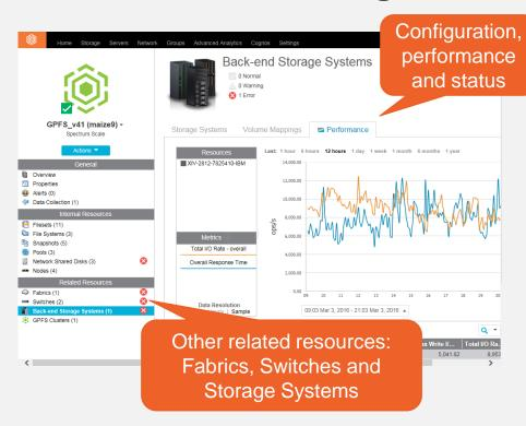
Clusters may use NSDs built off of SAN attached storage such as FlashSystems or other block storage systems. Latency within the Spectrum Scale file system may be due to issues within the storage or the fabric connections.
